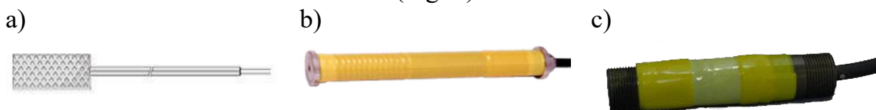
Figure 1. Embedded strain gauges: a - strain gauges of the KM-30-120-H1 series, b - strain gauge in concrete BS-25AT/BT, c - strain gauge in concrete BS-8FT (small)
