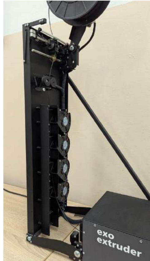
Fig. 10. Cooling and winding systems of composite threads
