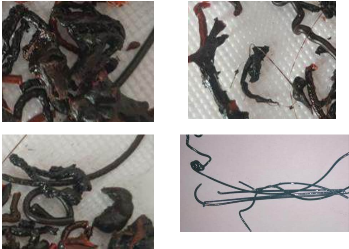
Fig.11. Polymer heating defects
