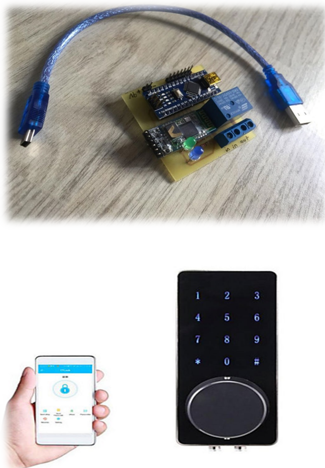
Figure 2: Hardware Architecture of the Bluetooth-Controlled Smart Door System
