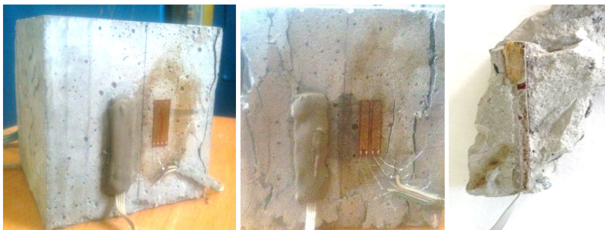
Figure 3. View of concrete cubes after testing
