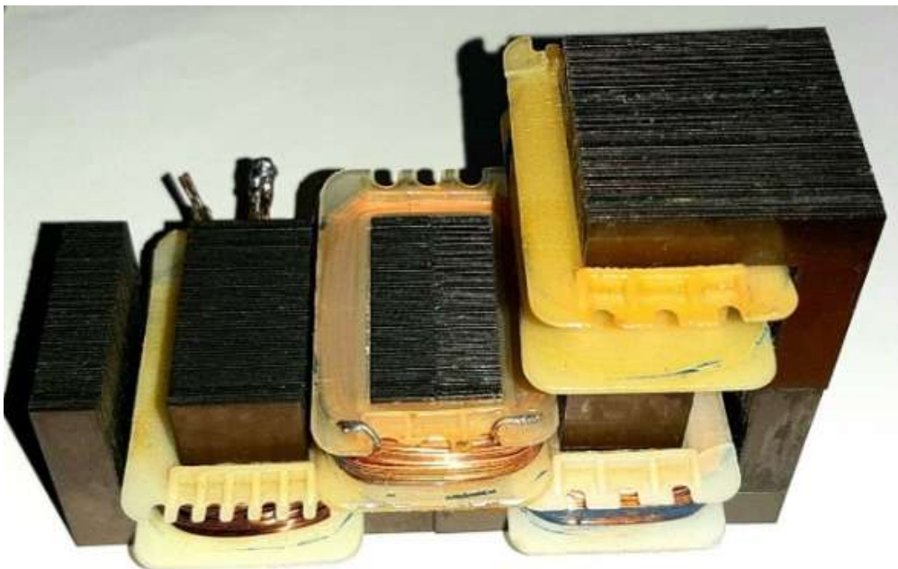
Figure 4 – Physical model of the inductor and stator section
