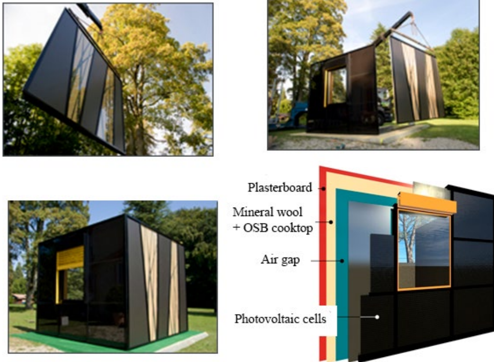
Pic. 7. Fast-moving buildings with photovoltaic modules Faceactive
